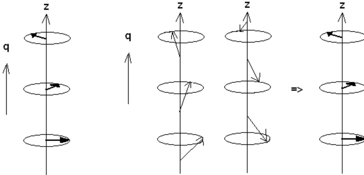
(Left) Plane spiral: Spins are almost exactly in the x-y plane. Large amplitude spiral, with large  $m_x$  and  $m_y$ , and  $m_z = 0$ . (see Herring: Bloch Wall)
